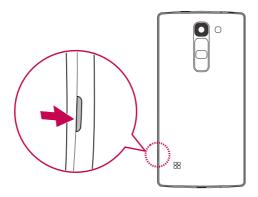
2 Slide the SIM card into the SIM card slot as shown in the figure. Make sure the gold contact area on the card is facing downward.
