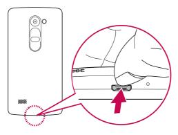
2 Slide the SIM card into the SIM card slot below the battery, as shown in the figure. Make sure the gold contact area on the card is facing downward.
