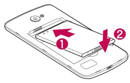
4 To replace the cover onto the device, align the cover over the back of the phoneand press it down until it clicks into place 2.
