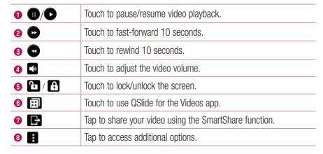
To change the volume while watching a video, press the Volume Up/Down Keys on the back of the phone.
