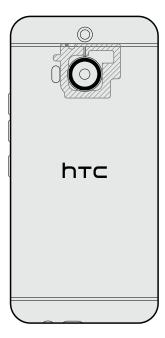
Make sure that the NFC area (shaded part) of HTC One M9+ and the other phone's NFC area are close to one another. Experiment by slightly moving the phones until a connection is made.
