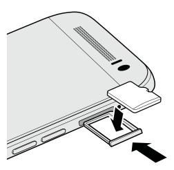
5. Insert the microSD card tray back into the slot.
