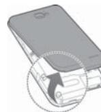
2. Insert the battery by aligning the contacts on the battery with the gold contacts in the battery compartment. Gently push down on the battery until it clicks into place.
