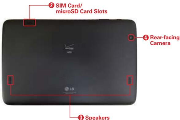
2. **SIM Card/microSD Card Slots** Use to insert your SIM card and a microSD card. A valid SIM card is required to have access to the mobile network. Insert an optional microSD card to store your personal data files (e.g., music, videos, photos, etc.).
