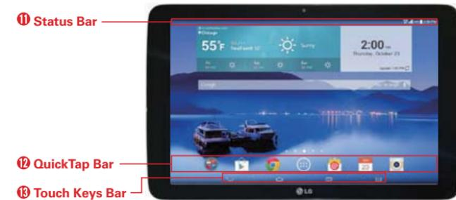
11. **Status Bar** Shows device information, including the time, status icons (such as signal strength, battery power, connections, etc.), and notification icons. It also provides access to the Notifications panel.
