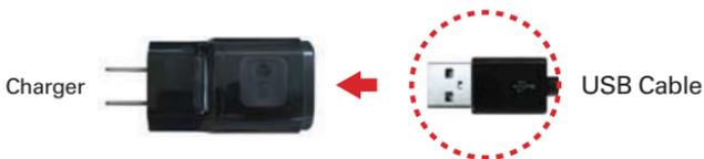
2. Insert the other end of the USB cable into the tablet's USB port.
