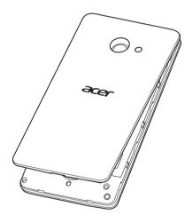
3. Insert the SIM or microSD card as shown.
