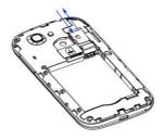
NOTE: The phone supports SD card hot-plug function. Some applications may require a microSD card to work normally or may store certain data on it. Therefore, it is recommended that you keep a microSD card installed and not remove or replace it randomly.
