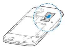
Some applications may require a microSDHC card to work normally or may store certain data on it. Therefore, it is recommended that you keep a microSDHC card installed and not remove or replace it randomly.
