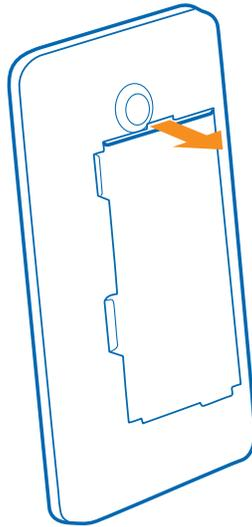
4. Push the SIM card into the SIM slot with the metal contact area down.
