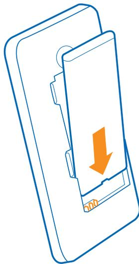
7. Press the bottom edge of the back cover against the bottom edge of your phone, and snap the cover into place.
