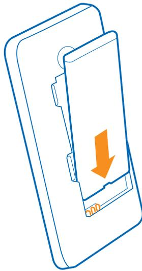
7. Press the bottom edge of the back cover against the bottom edge of your phone, and snap the cover into place. Don't press the keys while attaching the cover.
