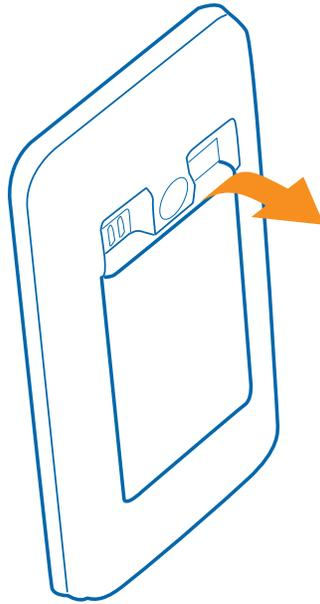
4. To remove the SIM card, pull it out from the slot.
