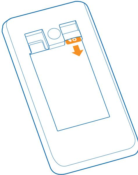
6. Line up the battery contacts, and put the battery in.
