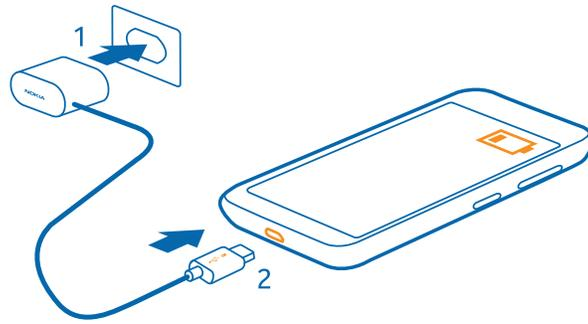
2. When the battery is full, disconnect the charger from the phone, then from the wall outlet.
