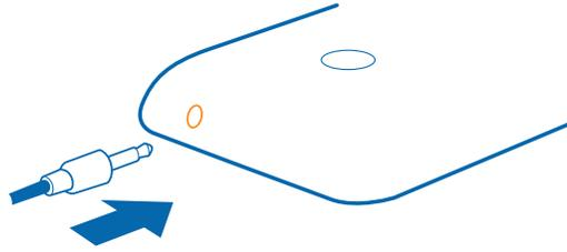
Do not connect to products that create an output signal, as this may damage the device. Do not connect any voltage source to the audio connector. If you connect an external device or headset, other than those approved for use with this device, to the audio connector, pay special attention to volume levels.
