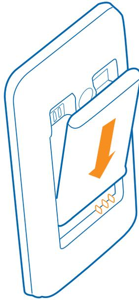
7. Press the bottom edge of the back cover against the bottom edge of your phone, and snap the cover into place. Don't press the keys while attaching the cover.
