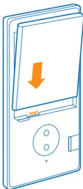
7. Press the top edge of the back cover against the top edge of your phone. Snap the cover into place, locking all the latches around the edges of the cover. Don't press the keys while attaching the cover.
