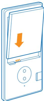
7. Press the top edge of the back cover against the top edge of your phone. Snap the cover into place, locking all the latches around the edges of the cover.
