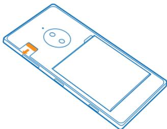
6. Line up the battery contacts, and put the battery in.
