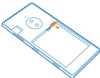
5. To remove the memory card, pull it out from the slot.
