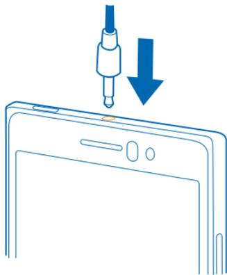
Do not connect to products that create an output signal, as this may damage the device. Do not connect any voltage source to the audio connector. If you connect an external device or headset, other than those approved for use with this device, to the audio connector, pay special attention to volume levels.
