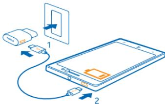
3. When the battery is full, disconnect the charger from the phone, then from the wall outlet.
