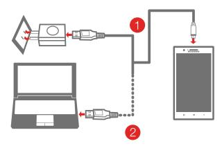
Method 1. Connect your smartphone to a power outlet using the cable and USB power adapter that come with your smartphone.
