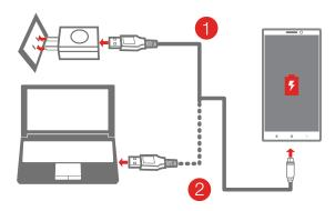
Method 1. Connect your VIBE to a power outlet using the cable and USB power adapter that come with your VIBE.
