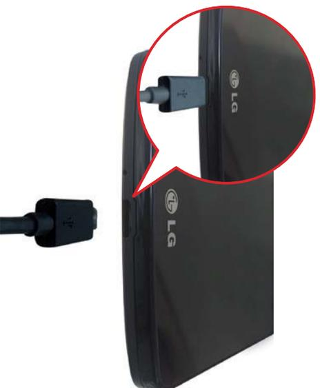
**WARNING!** To avoid damage to your phone's port and cable plug, orient the plug with the port before inserting it.
