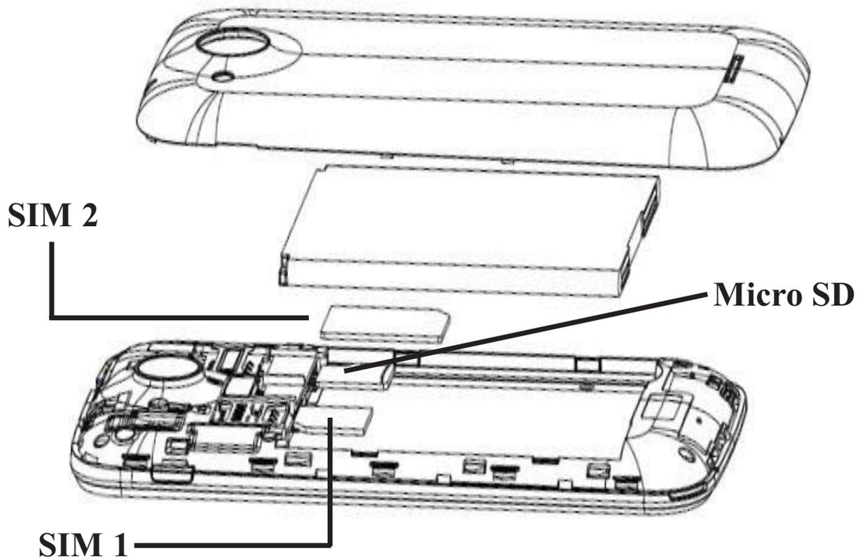
3. Finally insert the battery and replace the rear cover of the mobile phone.
