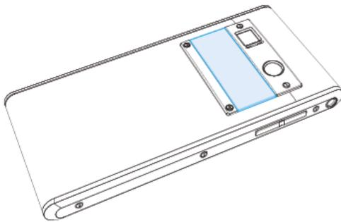
2. Next open the SIM door and place your microSIM into the cavity as shown.
