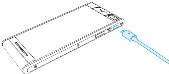
2. When the battery is fully charged, disconnect the charger from the phone and then from the wall outlet.
