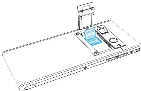
3. Finally, close the SIM door and lock into place (pictured). Then close the back cover and slide back.
