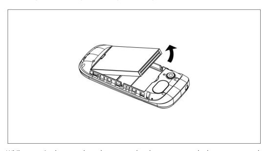
While removing battery, please bottom up the phones, remove the battery cover and pull the battery.
