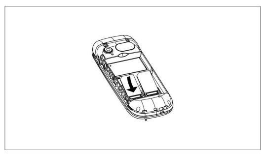
Put the SIM card into the card slot with copper sheet downward. When pull out the sim card, please power off the phone and connectors firstly.
