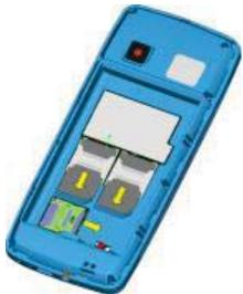
3) With the metallic contacts of the battery facing the metallic contacts in the battery slot, press the battery down until it locks into place, then fix its back cover.
