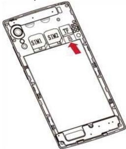
Finally replace the rear cover of the mobile phone. Use only compatible memory cards approved by with this device. Incompatible memory cards may damage the card or the device will corrupt the data stored in the card.
