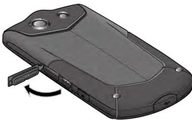
2. Carefully insert a microSD card into the microSD card slot on the left with the gold terminals facing down. Gently push the card into the slot and close the cover.
