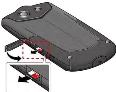
4. Press around the edges of the cover to the microSD card/SIM card slots to ensure that it is securely closed.
