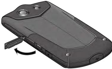
2. Carefully slide the SIM card into the SIM card slot on the right and close the cover.
