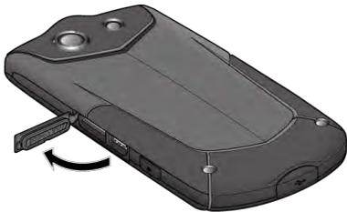
3. Push the SIM card gently with your finger. The card rejects itself. Pull out the card from the slot and close the cover.
