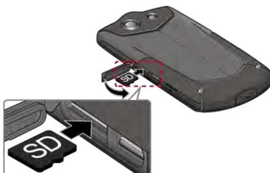
3. Press around the edges of the cover to the microSD card/SIM card slots to ensure that it is securely closed.
