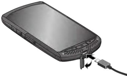
4. When charging is complete, remove the cable from the port and close the cover. Press around the edges of the cover to ensure that it is securely closed.
