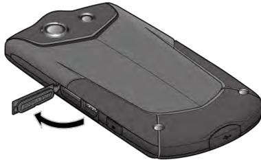
2. Push the microSD card and the card is partly ejected. Gently pull out the card from the slot and close the cover.
