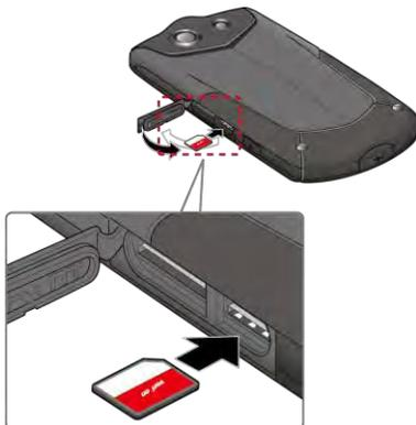
3. Press around the edges of the cover to the microSD card/SIM card slots to ensure that it is securely closed.
