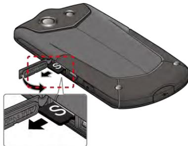
3. Press around the edges of the cover to the microSD card/SIM card slots to ensure that it is securely closed.
