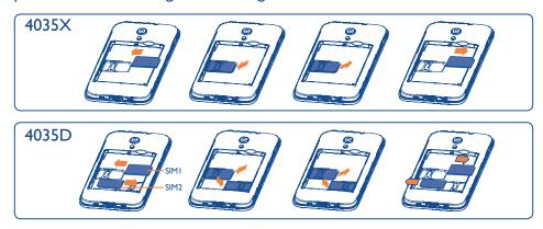
Place the SIM card with the chip facing downwards and slide it into its housing. Make sure that it is correctly inserted. To remove the card, press and slide it out.
