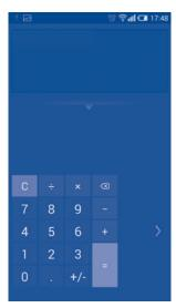
Enter a number and the arithmetic operation to be performed, enter the second number, then touch "=" to display the result. Touch to delete digits one by one, touch and hold to delete all at one time.
