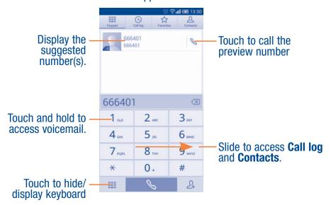
Enter the desired number from the keyboard directly or select a contact from **Contacts** or **Call log** by sliding or touching tabs, then touch to place the call.
