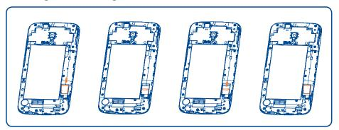
Insert the microSD card with golden contact facing downwards into the slot. To remove the microSD card, slide it out.
