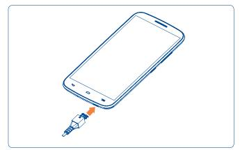
Connect the battery charger to your phone and main socket respectively, the LED indicator will light while charging.
