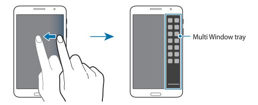
2 Tap and hold an application icon on the Multi Window tray, and then drag it to the screen. Release the application icon when the screen turns blue.
