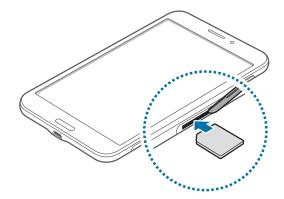
3 Push the SIM or USIM card into the slot until it locks in place.
