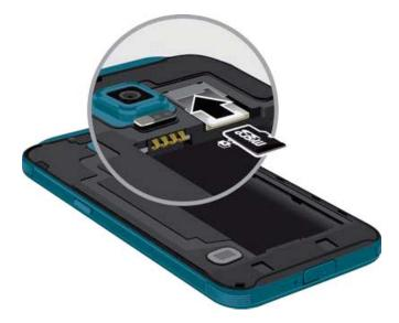
Carefully slide the memory card into the memory card socket (as shown) until the card locks into place. Make sure that the card's gold contacts face into the phone and that the card is positioned as shown.
