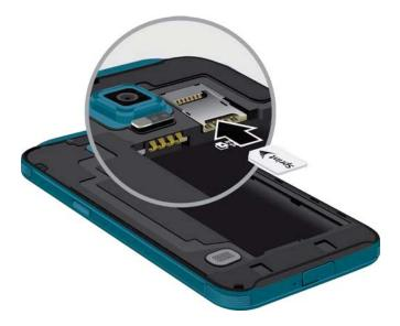
Carefully slide the SIM card into the SIM card socket (as shown) until the card locks into place.
