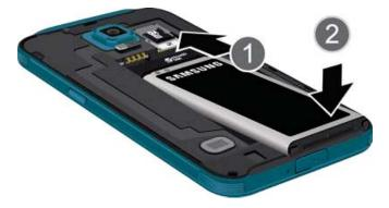
Insert the battery, aligning the gold contacts on the battery with the gold contacts on the phone, and gently press the battery into place.
