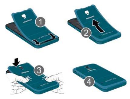
Replace the battery compartment cover, making sure all the tabs are secure and there are no gaps around the cover.
