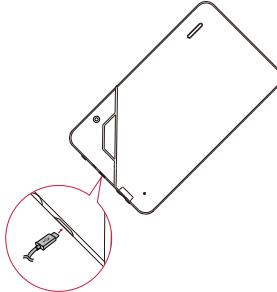
1. Plug the small end of the USB cable into the micro USB port of the device, and plug the large end of the cable into travel charger.
