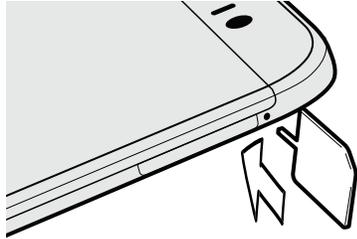
3. Push the tip all the way into the hole until the microSD card tray ejects.
