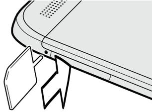
3. Push the tip all the way into the hole until the card tray ejects.
