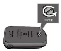
**Note:** The battery cover screw is permanently mounted on the cover and cannot be removed.
