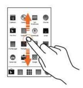
To scroll a list, slide your finger across the surface of the screen upwards or downwards (without dragging an item).
