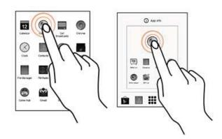
Tap and hold an item to view the list of actions based on the selected item and condition. Also, you can move an item from the apps screen to the home screen using this method.
