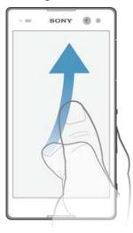
Scroll quickly, for example, in a list or on a web page. You can stop the scrolling movement by tapping the screen.
