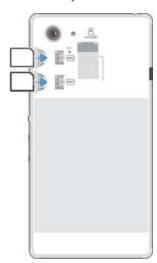
Remove the back cover, then insert the SIM cards into the corresponding slots with the gold-coloured contacts facing down.
