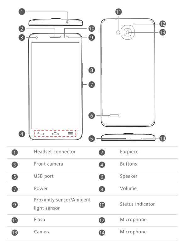
Do not block the area around the ambient light and proximity sensor. If you attach a protective film to the screen, make sure it does not block the sensor.
