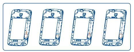
Insert the microSD card with the golden contact facing downwards into the slot. To remove the microSD card, slide it out.
