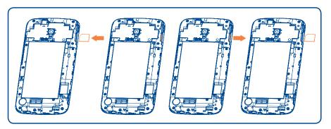
To install, place the SIM card with the chip facing upwards into the housing, and then slide it into its slot. Make sure that it is correctly inserted. To remove the card, press and slide it out.
