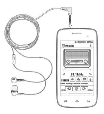
Press the phone's volume up/down keys on the right side of the mobile phone to adjust the volume.
