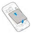
4. Align the back cover with the back of the phone and press the cover back into place. Make sure all the tabs are secure and there are no gaps around the cover.
