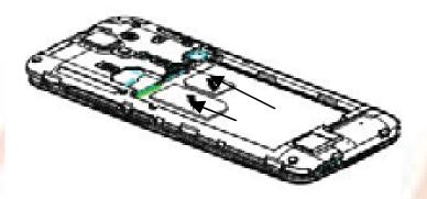
2. Finally insert the battery and replace the rear cover of the mobile phone.
