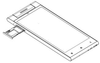
3. Push the Micro-SIM Box into the card slot.
