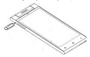
2. Insert the Micro-SIM card correctly in Micro-SIM Box.
