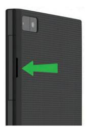
2. With the metal contacts facing you, insert the micro SIM card into the bottom slot.
