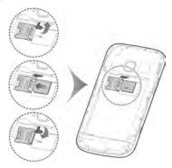
The microSDHC card can be installed and removed while the phone is turned on. Unmount the microSDHC card before removing it.
