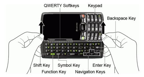
**Note:** When the slide-out keyboard is opened, the display stays in landscape mode and you can use the keypad on the front panel for entering numbers.
