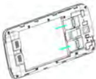
3. Insert memory card. Take compatible micro SD card, and place it into its respective slot.
