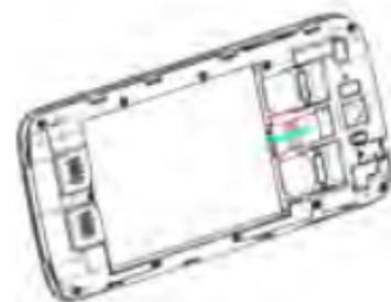
4. Replace the battery. Align the contacts of the battery with the corresponding connectors in the battery compartment & place the back cover.
