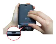
2. Insert the battery into the opening on the back on the phone, making sure the connectors align 1 and press down until it clicks into place 2.
