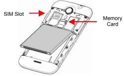
3. Insert the battery and replace the rear cover of the mobile phone.
