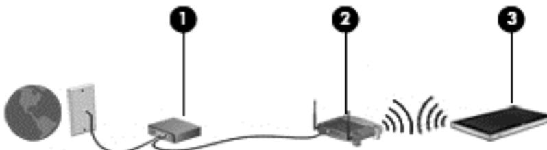
As your network grows, additional wireless and wired computers can be connected to the network to access the Internet.
