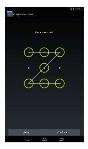
After you have set and activated the pattern unlock function, the unlock keypad will be displayed whenever the display is to be unlocked. Use your finger to trace your preset pattern on the keypad. After the preset pattern has been correctly entered, the screen will be unlocked.
