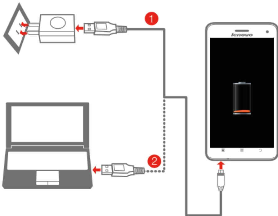
**Method 1.** Connect your phone to a power outlet using the included cable and USB power adapter.
