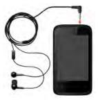
You will be required to plug in your headset before starting the FM Radio. The headset works as antenna for the FM radio.
