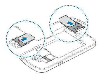
► Single SIM models: Pull out the SIM or USIM card.
