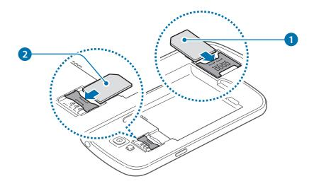
► Single SIM models: Insert the SIM or USIM card with the gold-coloured contacts facing downwards.
