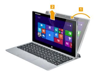
**Note:** Be careful not to damage the connector when attaching or detaching the tablet.
