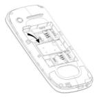
Note: The mobile phone does not support hot-plug function of T-FLASH in "power on" mode. Only when the mobile phone is powered off can T-FLASH be pulled out.
